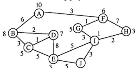
The numbers written on edges represent the distance between the nodes. The numbers written on nodes represent the heuristic value.
