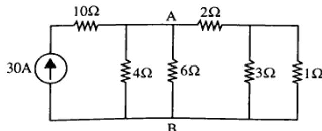
5. a) Find  $V_{ab}$  using Superposition theorem.
