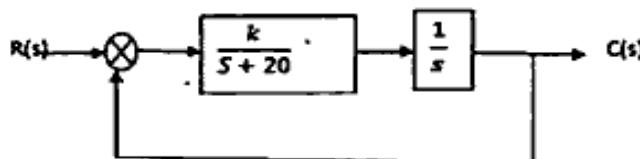
3. a) Explain time response of first order system to unit step and unit ramp input. Find the steady state error response for both.
